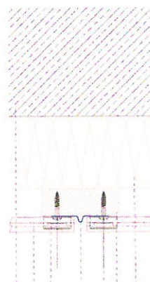
Horizontal cross-section connecting batten, screwed
